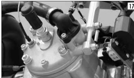
Check the level and proceed with the bleeding operation after having run the engine for the first time that must be done by connecting the choke wire to the carburetor. Connect the switch-off wire that comes out from the coil to an earth-connected switch. Then start the engine for a few seconds; stop the engine, check the level and if necessary top up with liquid.
