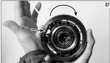
Now insert the plastic wheel in its housing again, and check through the hole that the internal spring hook is perfectly coupled (Photo 8),
