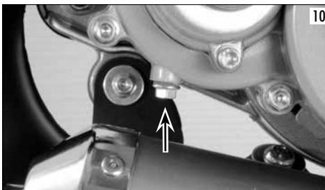
and collect the leaking liquid. Remove the cap to make this operation easier.
