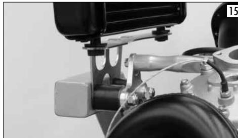
Fit the two rubbers on the bracket and place the radiator. To fix the radiator in the top side a bracket and a rubber are provided; the bracket has to be then connected to the frame using some brackets (not supplied)
