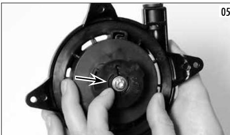
**⚠ Attention!** Under the cover there are two teeth for the starter jaw (check their condition and if worn replace them); under them 2 small calipers. Be very careful not to lose these small parts. Prepare the new rope and tie a knot at the top. Remove the plastic
