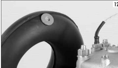
The EGT temperature detected in this position in standard conditions of use should be around 500°-620°, maximum temperature 650°.
