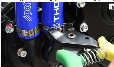
It is possible to place the radiator even in the bottom (see exploded view B). To facilitate the passage of the water tube on the head you have to use a special 90° connector - cod. 928.225.004 and 928.225.006 (not supplied). In this case you should be very careful to the position of the radiator that must have a proper housing and a strong fixing. Eventually place a breather pipe (928.225.006 and 928.225.004) to avoid air bubbles may start (see exploded view B).
