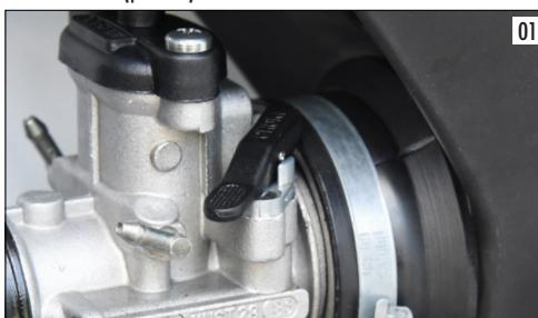
Operate the starter without accelerating till the engine starts. Once it runs switch it off, disconnect the starter and start the engine again slightly accelerating.
