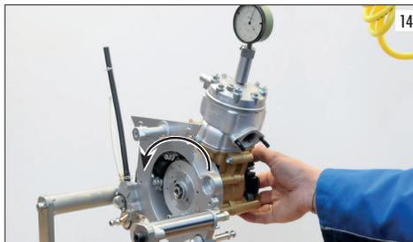
Once achieved the value, keep the pulley or the crankshaft stopped using one hand and tight the flywheel nut using a key, without exceeding. Check that the advance timing is as indicated (1,7+/- 0,1), remove the m.5x30 screw and fit the coil. Before locking it with the 2 screws, place between coil and flywheel one 0,35 mm calibrated shim (photo 15). Now definitely tight the flywheel nut using a torque wrench at 40Nm.
