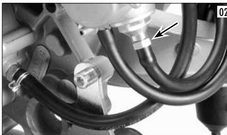
**⚠ ATTENTION:** never unscrew more than half a turn the breather nut to avoid damaging the OR seal. Never close too hard.
