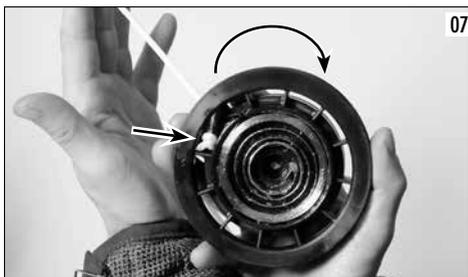
Now insert the plastic wheel in its housing again, and check through the hole that the internal spring hook is perfectly coupled (Photo 8), place the springs, the teeth for the starter jaw and screw the cover again using medium thread-locker. All the parts in movement, including the springs, must be well lubricated.
