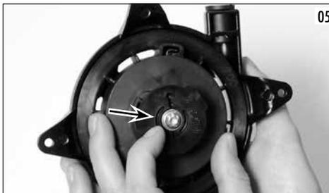
**⚠ ATTENTION!** Under the cover there are two teeth for the starter jaw (check their condition and if worn replace them); under them 2 small calipers. Be very careful not to lose these small parts. Prepare the new rope and tie a knot at the top. Remove the plastic wheel and the old rope. Thread the new rope in its hole (photo 6), wind up the rope on the wheel (according to the entrance sense of the rope on the wheel Photo 7).
