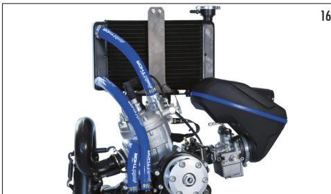
Fix the big bracket supplied between the two vibration-dumping mountings at the top and the frame. Fit the two rubbers on the bracket and place the radiator. To fix the radiator in the top side a bracket and a rubber are provided. Cut to size the water pipes and mount them. Close the supplied clamps using special pliers for its fitting (photo 17).
