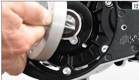
Screw the flywheel nut without locking it so that the crankshaft can rotate in the flywheel. Screw the dial gauge support into the spark plug hose, insert the dial gauge and move the piston to the top dead centre. Now reset the dial gauge and rotate the crankshaft anti-clock wise of X mm towards the flywheel sense (see arrow in photo 13).
